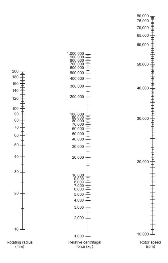
Centrifugation defines a relative centrifugal force (=RCF - measured in × g), corresponding to a speed (in rpm) for a particular centrifuge and a particular rotor. In many cases this nomogram substitutes for the equation:
